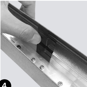
4 Attach strip of black tape to inside edge of housing
