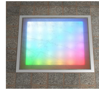
RAD 250 RGB video Buried uplight 36 x 1 Watt RGB LEDs Integral drivers 12 Volt - 48 Volt DC supply Artnet control Variety of diffuser options Stainless steel bezel Anti slip coating on glass IP 68
