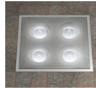
RAD 250 Buried uplight 4 x 15 Watt Xicato White LEDs Integral drivers 12 Volt - 48 Volt DC supply Variety of reflector options Stainless steel bezel Anti slip coating on glass IP 68
