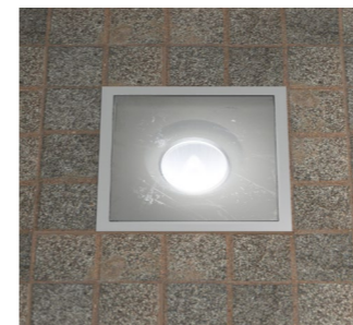
RAD 150 Buried uplight 1 x 23 Watt Xicato White LED Integral drivers 12 Volt - 48 Volt DC supply Variety of reflector options Stainless steel bezel Anti slip coating on glass IP 68
