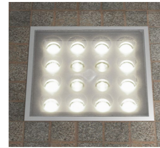
RAD 250 Buried uplight 16 x 3 Watt Cree XPE White LEDs Integral drivers 12 Volt - 48 Volt DC supply Variety of lens or reflector options Stainless steel bezel Anti slip coating on glass IP 68
