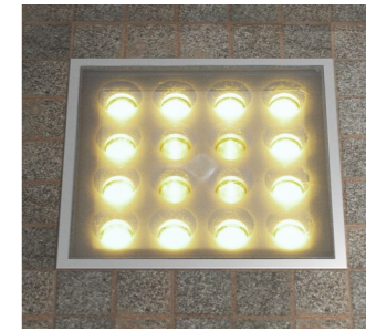
RAD 250 Buried uplight 16 x 3 Watt Cree XPE White LEDs With colour gel for fixed subtle colour tints. Refer to Rosco Supergel range for available colours. 12 Volt - 48 Volt DC supply Variety of lens options Stainless steel bezel Anti slip coating on glass
