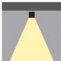
Interior - Surface Mounted Direct - Ceiling
