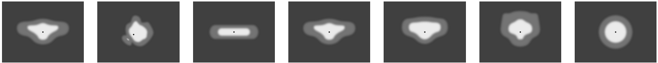
[T2] Type II, Asymmetric, Side throw [P4] Special pedestrian road distribution-right side traffic [T1] Type I, Asymmetric, Side throw [T2-2] Type II, Asymmetric, Side throw [T3] Type III, Asymmetric, Side throw [T4] Type IV, Asymmetric, Forward throw [T5] Type V, Symmetric
