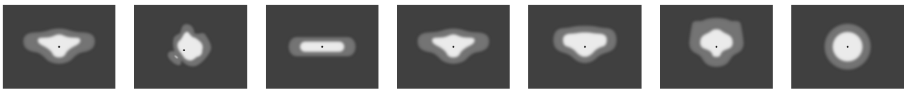
[T2] Type II, Asymmetric, Side throw [P4] Special pedestrian road distribution-right side traffic [T1] Type I, Asymmetric, Side throw [T2-2] Type II, Asymmetric, Side throw [T3] Type III, Asymmetric, Side throw [T4] Type IV, Asymmetric, Forward throw [T5] Type V, Symmetric
