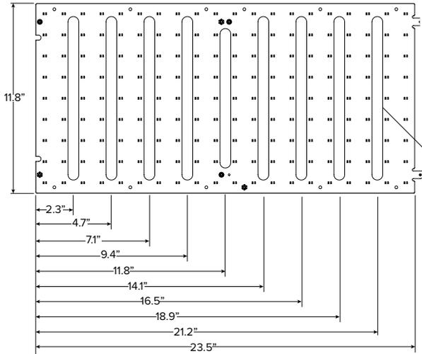
Slots to allow sound transmission to acoustic materials
